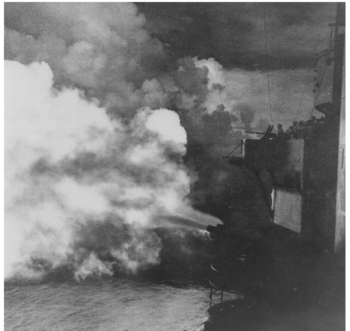
Shown here are the 14-inch 50 caliber guns of USS New Mexico being used to shell Guam on July 12, 1944. The heavy smoke is likely due to the effects of high humidity, worn barrels that caused incomplete powder combustion, and older barrel designs that burned powder less efficiently. (Official U.S. Navy Photo.)
