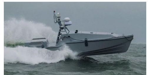
A Saronic Corsair 24-foot autonomous speed boat. Photo from Saronic Technologies, Austin, TX
