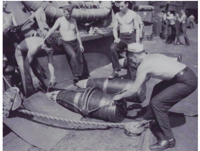
Shown here are sailors from USS New Mexico at Eniwetok in June of 1944. The sailors are preparing to lower 14-inch shells into the ammunition magazines of The Queen. These are likely 1,275 pound Mark 19 high explosive shells that were being loaded in preparation for the Battle of Guam. (Official U.S. Navy Photo.)
