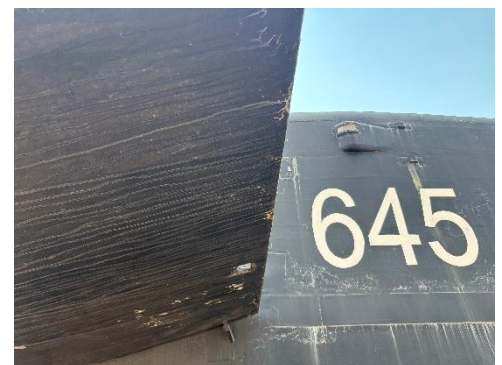
A unique perspective in this photo shows the underside of the bow planes attached to the sail. (Photo by Shelley Takeuchi)
