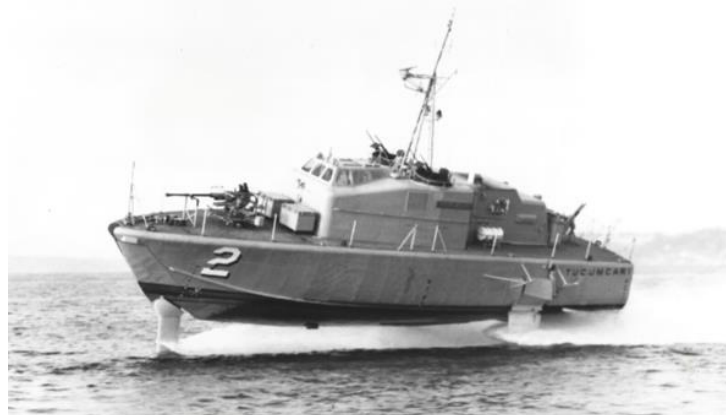
USS Tucumcari (PGH-2) in “flight.” The hydrofoil’s sailors used aviation terminology, including “take off,” “land,” and “fly.” (Boeing Company Photo).
